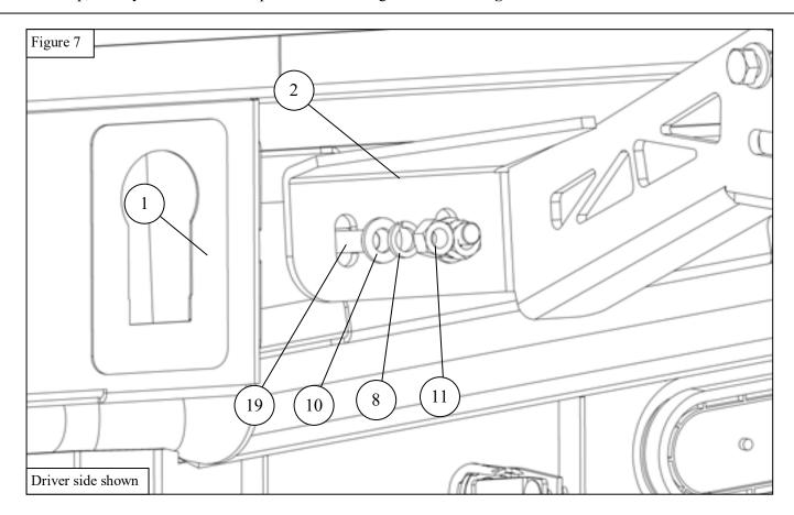
11. Install the Trailer plug and license plate at this time.
