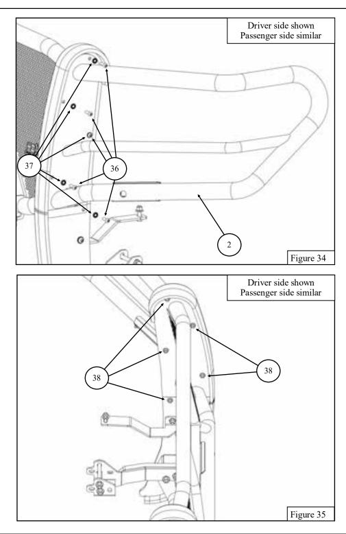
45. Align and adjust the Grille Guard Base, HDX Wings, and mounting brackets as necessary. Tighten and then torque all hardware as specified: M8 to 15-18 ft. lbs., M10 to 35-40 ft-lbs., and M12 to 55-60 ft-lbs.
