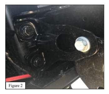
3. Loosely install the Driver and Passenger Mounting Brackets (Items 2-3) on to the inside of the frame reusing the factory hardware. See **Figure 3** for reference.
