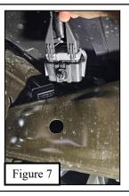
7. Detach the end of the wiring harness that is located in the inside of the bumper, see **Figures 8 & 9.**
