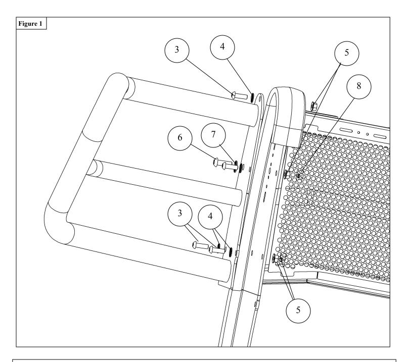
2. Adjust as needed and torque all hardware as specified: M10 to 35-38 ft-lbs., M12 to 50-55 ft-lbs.
