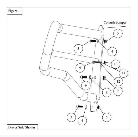
3. Adjust as needed and toque hardware as specified: M6 to 5-7 ft. lbs, M10 to 35 ft-lbs, M12 to 50 ft-lbs.
