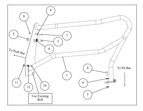
3. Adjust the wing wraps as needed and then tighten all hardware as specified: M6 to 8 ft-lbs. M8 to 20 ft-lbs. M12 to 60 ft-lbs.
