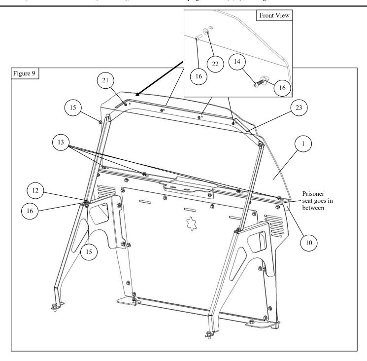
11. Adjust as needed and torque as specified: M6 to 5-7 ft. lbs. M8 to 15-18 ft. lbs., M10 to 35-38 ft lbs., M12 to 50 ft. lbs.
