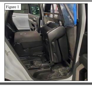
3. Locate the two rear holes on the floor for the upright brackets. Cut away enough rubber flooring just to access the holes. The front-most holes are 36.4 inches apart. The rear-most holes are 48 inches apart. *Note: if there are studs near the mounting holes, cut them off.* **See Figure 2-3**
