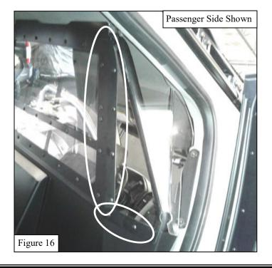
18. Align and adjust the Partition Assembly as needed. Torque all hardware as specified: M6 to 8 ft-lbs, M8 to 18 ft-lbs, M10 to 38 ft-lbs.
