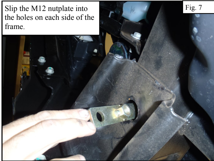
Partially thread this assembly into the nutplate.
