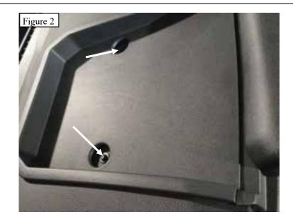
Place the Dash Mount Base (1) and align the slots with the dash board holes. Use two M5 long bolts (12), two 1/4" washer (9) and two 1/4" lock washer (8) to hold down the Dash Mount Base. Figures 3 and 4.
